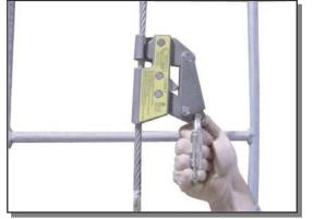
**Step 5:** Attach a CSA or an ANSI certified karabiner (according to the Jurisdiction) to the Slider. The attachment from the sternum D ring to the Slider should not exceed 0.15 M (6 in) in length. With the karabiner installed, the Slider cannot be removed from the cable. To ensure the Slider is functioning properly, pull down on karabiner to duplicate a fall arresting situation. Slider should grab the safety cable immediately.
