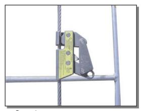
**Step 4:** The Slider should rest on the cable like this.
